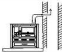
Wrong air flow caused by open doors on unused cooker
